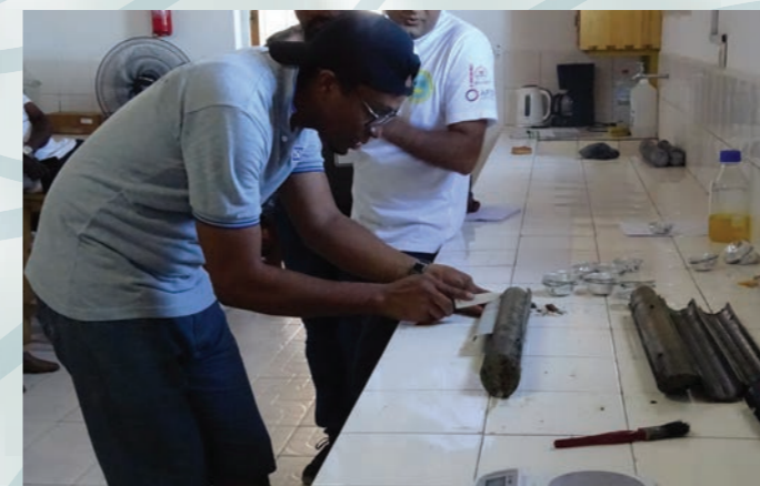
Preparing collected soil core samples collected in the laboratory - IORA Training Workshop on Blue Carbon Research, Madagascar.
